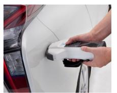
The compact body (with hand strap) can be stably held with one or two hands. Moreover, it is loaded with features ideal for measuring vehicle exteriors such as a rubber cover around the measurement aperture to safeguard measurement subjects against scratching and Bluetooth® support (option) for sending measurement data to remote devices over wireless connections.
